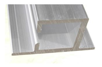
The heart of every aluminum enclosed gate track system is the track assembly. Our standard track length is 31 feet. It is extruded of high quality aluminum and then heat treated. The back flange can be easily drilled to mount to a standard pipe cantilever gate or may be welded to an aluminum frame gate. We manufacture a heavy duty extrusion to add strength to the gate. Heavier one piece extrusions are better.
