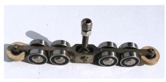
This is our new heavy duty 8 roller aluminum track trolley. The mounting bolt is a rod end that self levels the trolley in relation to the to the aluminum track assembly. This allows smoother gate operation and roller efficiency. The chassis is made of forged stainless steel.
